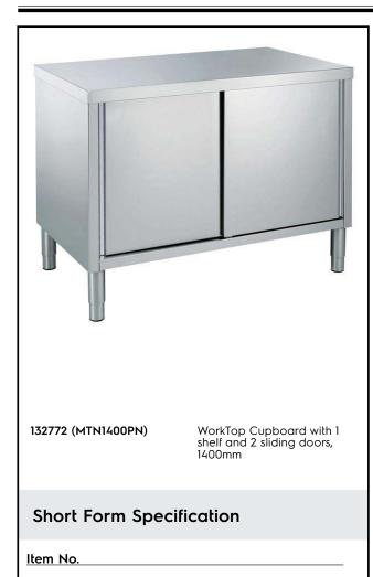
Made entirely from stainless steel. Inner welded frame in stainless steel. Unique connection of panels to inner frame. The 50mm high worktop in 304 AISI stainless steel, 1mm in thickness, incorporates a layer of sound deadening material and has upturned edges. Sound-deadened sliding doors. Base panel in 304 AISI stainless steel and heightadjustable intermediate shelf. Mounted on feet, adjustable in height.
